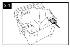
**d.** Remove lint from filter screen located inside recovery tank.
