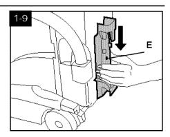
Slide rack down into place. Insert screw at (E) and tighten with a Phillips screw-driver.
