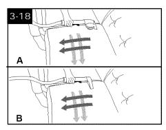
necessary to repeat the cleaning process. Make crisscrossing strokes to the original pattern; overlap each pass.
