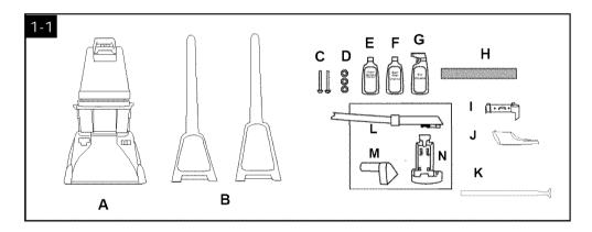
Unpack deep cleaner from the carton and identify the parts shown. Remove and dispose of the packing.
