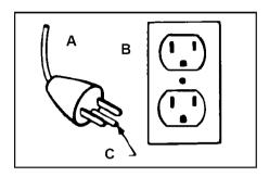
This appliance must be grounded. If it should malfunction or breakdown, grounding provides a path of least resistance for electrical current to reduce the risk of electric shock. This appliance is equipped with a cord having an equipment-grounding conductor (C) and grounding plug (A). The plug must be plugged into an appropriate outlet (B) that is properly installed and grounded in accordance with all local codes and ordinances.
