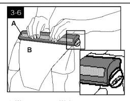
2. With foam strip (A) (located under the netting) in position as shown, place attachment on front of nozzle (B).
