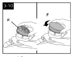
seconds). Then squeeze the trigger and begin cleaning.
