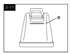
Pour detergent into tank. Fill tank to fill line (B) (1 gallon) with hot tap water.
