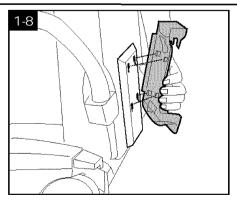
Attach tool holder Remove tool and taped screw from holder.
