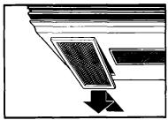
2. To remove grease filters, slide each filter to the front.
