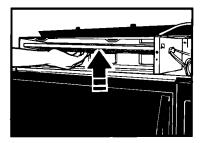
Lift the back of the charcoal filter. Slide the filter straight out.
