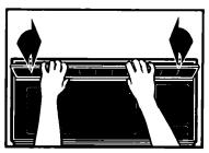
Slide the bottom of the vent cover into place.
