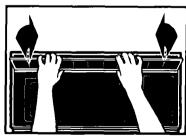
8. Silde the top of the vent cover into place. Push the bottom until it snaps into place. Replace the mounting screws. Turn the power back on at main power supply.
