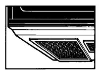
**11.** Do not operate the hood without the filters in place.
