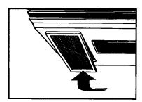
**4. To replace grease filters,** slide filter in the frame slot on the front of the opening.
