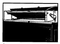
**8.** Slide a new charcoal filter into place. The filter should rest at the angle shown.
