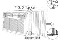
Your air conditioner is designed to install in standard double hung windows with opening widths of 23 to 36 inches (584 mm to 914 mm) (FIG. 4A, FIG. 4B).
