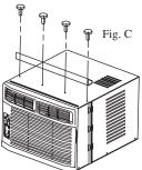
NOTE: FOR SAFETY REASONS, ALL FOUR (4) SCREWS <u>MUST</u> BE SECURELY FASTENED.
