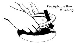
2. Line up opening in the reflector bowl with the surface unit receptacle.
