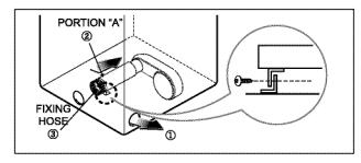
3. Reconnect the new duct[11 in(28cm)] to the blower housing, and Fixing the duct to the base.
