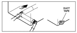
${\bf 5.}$  Insert duct assembly, elbow first, through the side opening and connect the elbow to the dryer internal duct.
