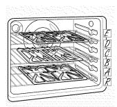
The oven has 5 rack positions. Place the gray porcelain-coated racks in positions "R", "B" and "D" for self-cleaning the grates. Place one grate each on the oven racks from side to side.
