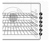
When convection baking with only 1 rack, follow the rack positions recommended in the Using the Oven section.
