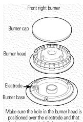
the burner head is fully inserted inside the burner base. A small gap between the base and head is normal.
