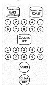
The upper oven will turn on immediately and cook for a selected length of time. At the end of the cooking time, the oven will turn off automatically.
