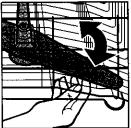
freely. Check the lower spray arm also to make sure it turns freely.
