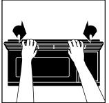
Push the bottom until it snaps into place. Replace the mounting screws.
