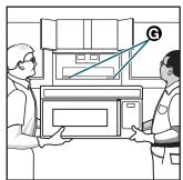
microwave oven downward. (Be careful that door does not swing open.) Lift off the support tabs () at the bottom of the mounting plate. Set the microwave oven aside on a protected surface.
