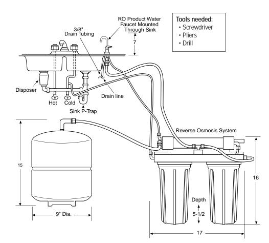
**Note:** Can be installed undercounter (as shown), in basement, or other convenient location. See installation instructions packed with product for complete details.
