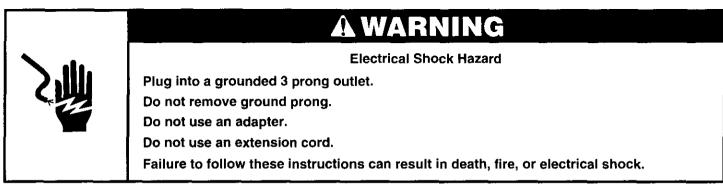
120-volt, 60-Hz., AC-only, 15- or 20-ampere fused electrical supply is required. (Time-delay fuse or circuit breaker is recommended.) It is recommended that a separate circuit serving only the clothes vitalizer be provided.
