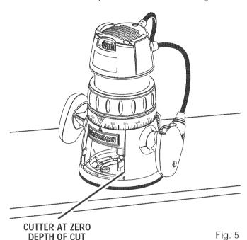
■ Position router so that the cutter can extend below the subbase for desired depth setting. See Figure 6.
