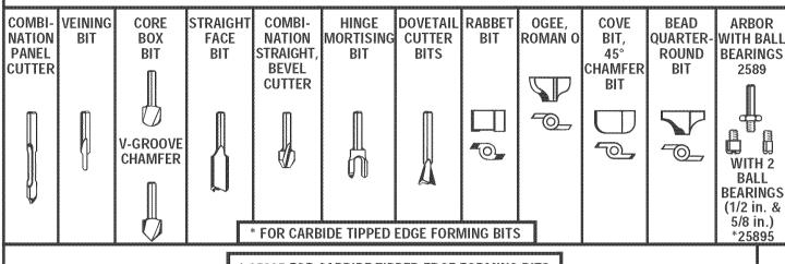
\* 25895 FOR CARBIDE TIPPED EDGE FORMING BITS 2589 FOR HIGH SPEED STEEL EDGE FORMING BITS
