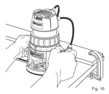
Rout the pattern in two or more passes. Make the first pass at 25% of the desired depth of cut. This will provide better control as well as being a guide for the next pass.
