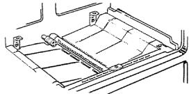
To determine if the bottom burner flames are burning properly, remove the oven bottom. Flames should have approximately 1" blue cones and, if range is supplied with natural gas, should burn with no yellow tipping. (With most LP gas, small yellow tips at the end of outer cones are normal.) Flames should not lift off burner ports. If lifting is observed, gradually reduce air shutter opening until flames are stabilized.
