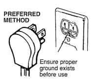
The customer should have the wall receptacle and circuit checked by a qualified electrician to make sure the receptacle is properly grounded.
