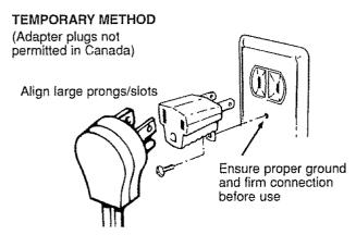
An adapter may be used only on a 15-amp circuit. Do not use an adapter on a 20-amp circuit. Where local codes permit, a **TEMPORARY CONNECTION** may be made to a properly grounded two-prong wall receptacle by the use of a UL-listed adapter, available at most hardware stores. The larger slot in the adapter must be aligned with the larger slot in the wall receptacle to provide proper polarity in the connection of the power cord.
