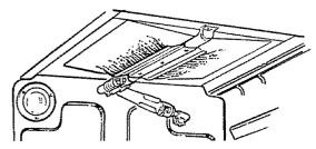
The flames for the top (broil) burner should burn steady with approximately 1" blue cones and should not extend out over the edges of the burner baffle.
