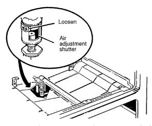
The shutter for the bottom (oven) burner is near the back wall behind the broiler drawer, WARM-N-READY drawer, storage drawer, or kick panel (depending on the model). Remove the drawer or panel. See the Care and Cleaning section in this guide.
