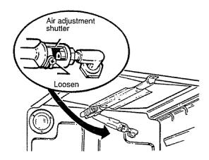
The air adjustment shutter for the top (broil) burner is in the center of the rear wall of the oven.
