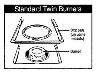
Your range is equipped with one of the two types of surface burners shown at left.
