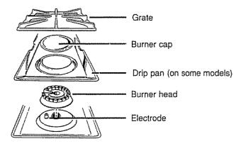
Turn all controls off before removing burner parts and drip pans (if so equipped).
