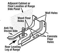
3. For wood construction, drill a ½" pilot hole in the center of each of the pre-marked wood floor and wall hole positions (a nail or awl may be used if a drill is not available). Fasten the Anti-Tip device with the 4 screws provided.
