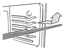
facing up and toward the rear of the oven. Tilt up the front and push the shelf toward the back of the oven until it goes past the bump on the shelf support. Then lower the front of the shelf and push it all the way back.
