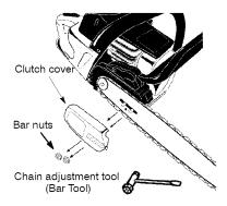
Turn adjusting screw on bar counterclockwise to move the tensioning rack as far as it will go toward the front of the bar.
