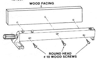
5 MITER GAUGE ... head is locked in position for crosscutting or mitering by tightening the lock knob. ALWAYS LOCK IT SECURELY WHEN IN USE.
