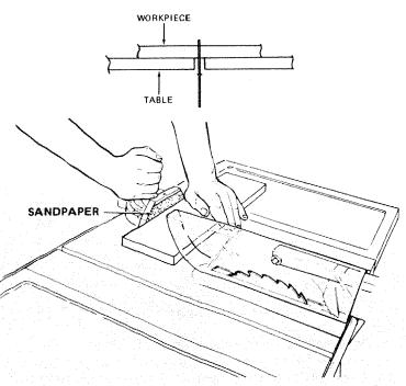
groove, hold the workpiece firmly against the miter gauge head with your left hand, and grip the lock handle with your right.
