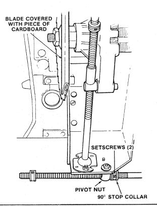
TILT blade to LEFT as far as it will go. It will stop when the PIVOT NUT is against the 45° STOP COLLAR.
