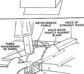
WING NUT SPREADER SPREADER CLAMP BRACKET
