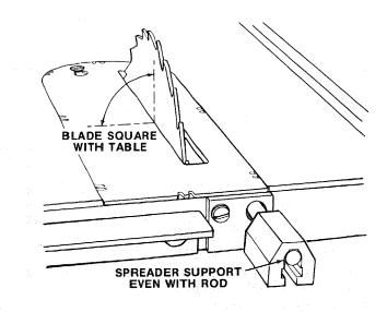
2. Position SPREADER SUPPORT on rod until it is even with the end of the rod.
