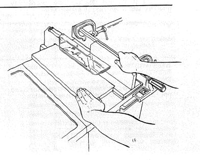
Narrow strips thicker than the Auxiliary Fence/Work Support may enter the guard and strike the baffle. CAREFULLY raise guard only enough to clear the workpiece. Use PUSH BLOCK to complete cut.
