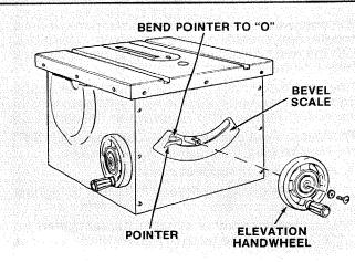
If blade is NOT SQUARE to table . . . the 90° LIMIT STOP must be ADJUSTED.
