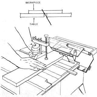
made at an angle other than 90° to both the edge and the flat side of the wood.
