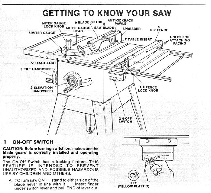
Do not cycle the motor switch on and off rapidly, as this may cause the sawblade to loosen. In the event this should ever occur, allow the sawblade to come to a complete stop and retighten the arbor nut normally, not excessively. Never leave the saw while the power is "ON".
