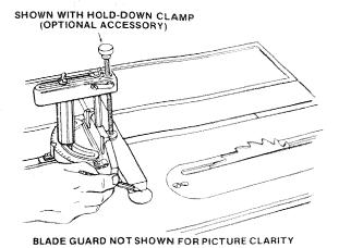
F. When cutting the workpiece, line up mark on workpiece with line on disc.
