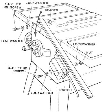
7. Insert one inch long screws in first and third holes of the rear guide bar and attach to table the same way as the front bar.
