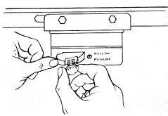
WARNING: FOR YOUR OWN SAFETY, LOWER BLADE OR OTHER CUTTING TOOL BELOW TABLE SURFACE. (IF BLADE IS TILTED, RETURN IT TO VERTICAL (90°) POSITION). ALWAYS LOCK THE SWITCH "OFF". WHEN SAW IS NOT IN USE ... REMOVE KEY AND KEEP IT IN A SAFE PLACE ... ALSO ... IN THE EVENT OF A POWER FAILURE (ALL OF YOUR LIGHTS GO OUT) TURN SWITCH OFF ... LOCK IT AND REMOVE THE KEY. THIS WILL PREVENT THE SAW FROM STARTING UP AGAIN WHEN THE POWER COMES BACK ON.
