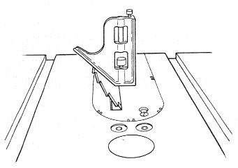
If blade is NOT 45° to table . . . the 45° STOP COLLAR must be ADJUSTED
