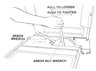
D. TO TIGHTEN nut . . . HOLD ARBOR wrench against rear of table . . . PUSH ARBOR NUT wrench toward rear.
