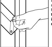
included with your range, into both hinge hangers. **Do not remove** the pins while the door is removed from the range.
