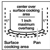
cooktops. Canners with rippled or ridged bottoms do not allow good contact with the surface.
