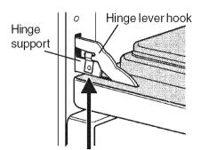
Lock engaged for door removal Figure 1
