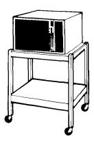
2. Put the oven on a cart, counter, table or shelf that is strong enough to hold the oven and the food and utensils you put in it. (The control side of the unit is the heavy side. Use care when handling.) The weight of the oven is approximately 70 lbs. (31.75 kg).
