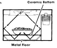
The ceramic bottom of your microwave oven lets microwaves through. Then they bounce off a metal floor, back through the ceramic bottom and are absorbed by the food.
