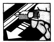
9. Move the Lock Lever back to the left. Do not force it. Wait until it will move easily. This turns off the Clean Light.
