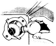
3. Remove the light bulb from its socket.
