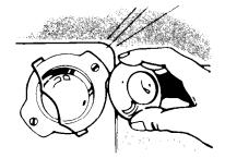
2. Remove the bulb cover by pulling out on the wire holder and moving it to the side.
