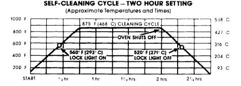
Notice that the heating stops when the two-hour setting is up, but that it takes a while longer for the oven to cool down enough to unlock.
