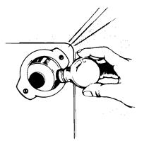
2. Remove the light bulb from its socket.
