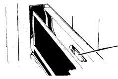
When the upper oven is on, hot air and moisture escape through a vent on top of the control panel. Air from the lower oven vents just above the lower oven door. These vents are needed for air circulation.
