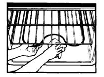
**10.** After the oven is cool, wipe off any residue or ash with a damp cloth. If needed, touch up spots with cleanser or soapy steel-wool pad.
