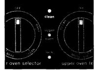
8. When the Lock Light goes off, turn the Upper Oven Selector and Temperature Control to OFF.
