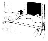
Lift **the cool bake element** slightly to lift the feet off the oven bottom.
