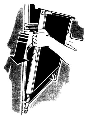
Push the door down evenly. The door will close only when it is on the hinges correctly.
