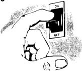
1. Turn off the electric power at the main power supply.
