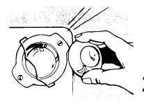
Replace the bulb cover and snap the wire holder in place. The bulb must have this cover when the oven is being used.
