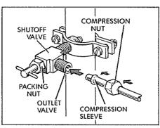
6. Slip compression sleeve and compression nut on copper tubing as shown above. Insert end of tubing into outlet end squarely as far as it will go. Screw compression nut to outlet end with adjustable wrench. Do not overtighten. Turn ON main water supply and flush out tubing until water is clear. Turn OFF shutoff valve on water pipe. You are now ready to connect other end of 1/4" copper tubing to water valve on back of refrigerator.
