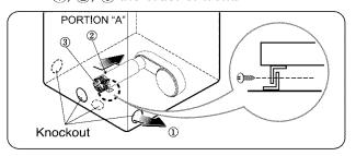
**2-2.** Reconnect the duct to the blower housing and attach the duct to the base.(Duct is a SVC part)
