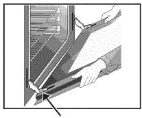
**HINGE SLOT-Door removed** from the appliance
