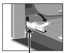
Lock engaged for door removal
