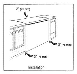
NOTE: The exterior walls of the freezer may become quite warm as the compressor works to transfer heat from the inside. Temperatures as much as 30° F warmer than room temperature can be expected. For this reason it is particularly important in hotter climates to allow enough space for air circulation around your freezer.
