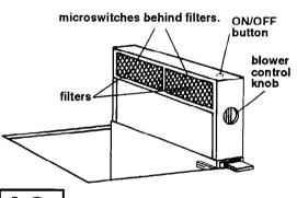
Turn power supply on. Push the button on the top of the downdraft vent. Retractable section of downdraft vent will rise and blower will start. Turn the control knob on side of vent to check the operation and speed of blower. If blower does not operate:
