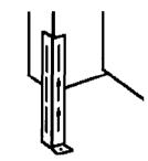
**5.** Move support legs down against cabinet floor. Place a level against front of downdraft vent base and adjust position of legs until downdraft is level vertically. Use a pencil to mark the top of each leg on face of downdraft vent. Then mark location of support leg mounting holes on cabinet floor. Remove downdraft vent from cutout. Drill starter holes at each mounting screw location on cabinet floor. Align top of legs with pencil marks on face of downdraft vent. Tighten screws in legs.
