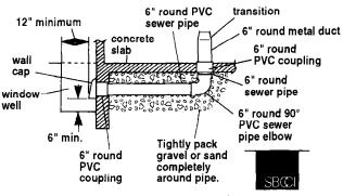
Seal the space between the outside of wall cap inlet inside of PVC coupling with caulking metal.
