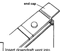
9. Insert downdraft vent into countertop cutout. Two people are recommended to support the weight of the downdraft vent during lifting. Position downdraft vent so it is centered in cutout and parallel to edge of cutout. Check that downdraft vent is level vertically. Then fasten lower support legs to cabinet floor with screws. Snap end caps over top of mounting brackets.
