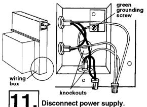
Thread the power supply cable through the knockout opening in the wiring box. Connect the white wires together with a twist-on wire connector. Connect the black wires together with a twist-on wire connector. Attach the green (or green and yellow) grounding wire to evelet with green grounding screw. Reattach the wiring box cover.
