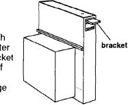
Attach support legs to side of downdraft vent with two screws in each leg. Do Not tighten screws.
