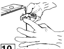
Attach one undercounter mounting bracket on front upper right corner of downdraft vent with slot over vent mounting hole and flange against countertop. Attach other bracket to left side of downdraft vent. Carefully drill starter holes through undercounter mounting brackets into underside of countertop. Insert appropriate length screws into holes and tighten brackets to countertop.
