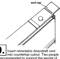
into countertop cutout. Two people are recommended to support the weight of the downdraft vent during lifting. Position downdraft vent so it is centered in cutout and parallel to edge of cutout. Check that downdraft vent is vertical. Then attach lower support legs to cabinet floor with screws. Snap end caps over top of mounting brackets.
