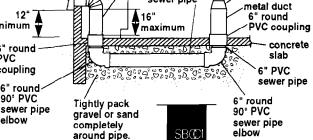
Optional ductwork installed under a concrete slab into a window well.
