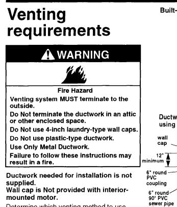
Determine which venting method to use. Ductwork can extend either through the wall or roof.
