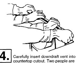
recommended to support the weight of the downdraft vent during lifting. Check that
