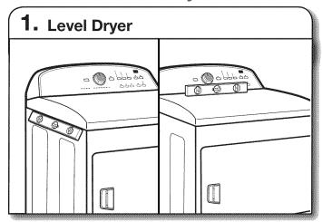
Check levelness of dryer from side to side. Repeat from front to back.
