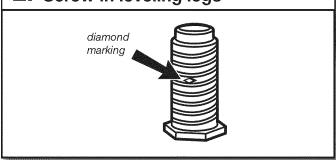
Examine leveling legs, find diamond marking. Screw legs into leg holes by hand, use a wrench to finish turning legs until diamond marking is no longer visible.
