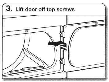
Lift door until top screws in dryer cabinet are in large part of hinge slot. Pull door forward off screws. Set door (handle side up) on top of dryer. Remove top screws from dryer cabinet.
