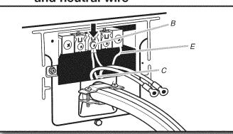
Connect neutral ground wire (E) and neutral wire (white or center wire) (C) of power supply cord or cable under center, silver-colored terminal block screw (B). Tighten screw.
