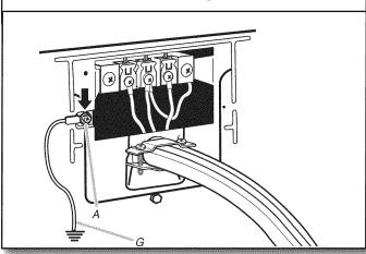
Connect a separate copper ground wire (G) from the external ground conductor screw (A) to an adequate ground. Finally, reinsert tab of terminal block cover into slot of dryer rear panel. Secure cover with hold-down screw. **Now, go to Venting Requirements.**
