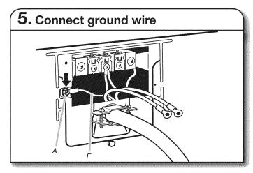
Connect ground wire (F) (green or bare) of power supply cord to external ground conductor screw (A). Tighten screw.
