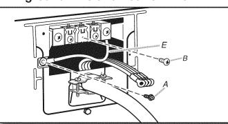
Remove center, silver-colored terminal block screw (B). Remove neutral ground wire (E) from external ground conductor screw (A).
