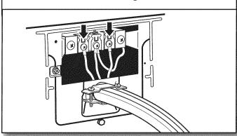
Place hooked ends of remaining wires under outer terminal block screws (hooks facing right). Tighten screws.
