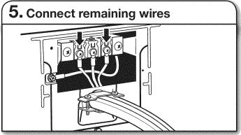
Connect remaining wires to outer terminal block screws. Tighten screws. Finally, reinsert tab of terminal block cover into slot of dryer rear panel. Secure cover with hold-down screw. Now, go to Venting Requirements.
