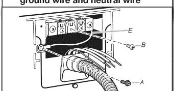
Remove center, silver-colored terminal block screw (B). Remove neutral ground wire (E) from external ground conductor screw (A).
