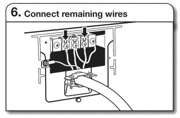
Connect remaining wires to outer terminal block screws. Tighten screws. Finally, reinsert tab of terminal block cover into slot of dryer rear panel. Secure cover with hold-down screw. Now, go to Venting Requirements.
