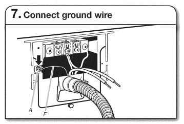
Connect ground wire (green or bare) (F) of direct wire cable to external ground conductor screw (A). Tighten screw.
