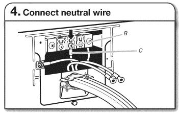
Connect neutral wire (white or center) (C) of power supply cord to center, silver-colored terminal block screw (B). Tighten screw.
