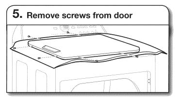
Remove screws at top, bottom, and side of door (5 screws). Keep door screws separate from hinge screws as they are different sizes. Holding door over towel on dryer, grasp sides of outer door and lift to separate it from inner door.
