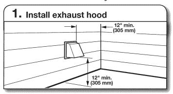
Install exhaust hood and use caulking compound to seal exterior wall opening around exhaust hood.
