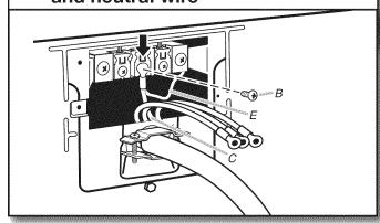
Connect neutral ground wire (E) and neutral wire (white or center) (C) of power supply cord under center, silver-colored terminal block screw (B). Tighten screw.
