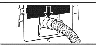
Put direct wire cable through the strain relief. The strain relief should have a tight fit with the dryer cabinet and be in a horizontal position. Tighten strain relief screw against the direct wire cable.
