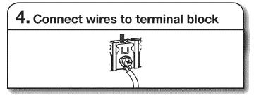
To connect wires to terminal block, place hooked end of wire under terminal block screw, facing to the right, squeeze hooked end together and tighten screw.
