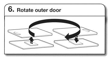
Take outer door and rotate it 180° and set it back down on inner door. Be certain to keep cardboard spacer centered between doors. Reattach outer door panel to inner door panel so handle is on the side where hinges were just removed. Insert 5 door screws.
