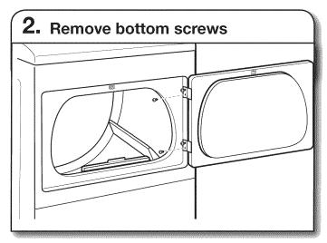
Open dryer door. Remove bottom screws from dryer cabinet side of hinges. Loosen (do not remove) top screws from dryer cabinet side of hinges.
