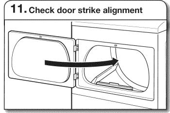
Close door and check that door strike aligns with door catch. If it is needed, slide door catch left or right within slot to adjust alignment.
