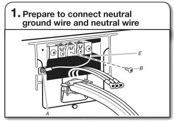
Remove center, silver-colored terminal block screw (B). Remove neutral ground wire (E) from external ground conductor screw (A).
