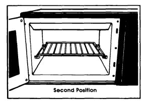
Note: Do not store the metal rack in the oven. Arcing and damage to the oven can result if someone accidentally starts the oven.
