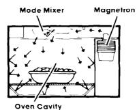
A magnetron in the microwave oven produces microwaves. The microwaves move into the oven where they are scattered or stirred by a mode mixer (like a fan). Microwaves bounce off metal oven walls and are absorbed by food
