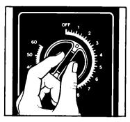
2. Set cooking times up to 60 minutes by turning the Timer Knob clockwise. To reduce the cooking time, turn the Timer Knob counterclockwise. Each mark represents 30 seconds for the first 10 minutes. For times longer than 10 minutes, each mark represents 2 minutes.
