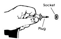
2. Place food in the oven and plug the probe into the socket on the oven wall
