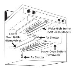
oven front frame, and pull the oven bottom out of the oven. Remove burner baffle so that the burner flame can be observe.
