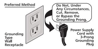
and circuit checked by a qualified electrician to make sure the receptacle is properly grounded and polarized.
