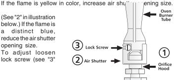
illustration below), reposition air shutter, and tighten lock screw. Replace oven bottom.
