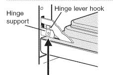
Lock engaged for door removal Figure 1
