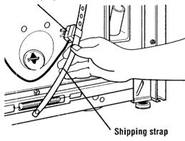
STEP 4. Cut the shipping strap about 16 inches from plug end. Look for the words "CUT HERE." Discard end with three cotter pins. Slide remainder of shipping strap free from the electrical plug. You will use this to secure the drain hose.
