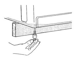
**STEP 4.** Tilt washer backward until front of washer is off the wood block. Remove wood block. Gently lower washer to floor.
