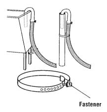
If the water faucets and drain standpipe are recessed, put hooked end of drain hose in standpipe. Tightly wrap the shipping strap around the drain hose and water inlet hoses (not the handles or stems). Push fastener into the nearest hole in the shipping strap.
