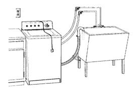
STEP 2. Locate the remaining piece of shipping strap (not the end with the three cotter pins) from STEP 4 of "REMOVE SHIPPING STRAP." Use it to wrap the drain hose together with the laundry tub or standpipe. Push fastener into the nearest hole in the shipping strap.
