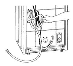
**STEP 3.** Insert one new, flat washer (from the parts bag) into each end of the inlet hoses. Check that washers are firmly seated in couplings.
