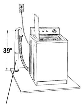
Standpipe drain system: Needs a two-inch minimum diameter standpipe with minimum carry-away capacity of 17 gallons per minute. Top of standpipe must be at least 39 inches above floor and no higher than 96 inches from bottom of washer.
