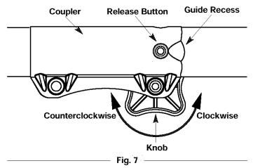
**NOTE:** Aligning the release button with the guide recess will help installation (Fig. 7).
