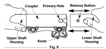
4. Turn the knob clockwise to tighten (Fig. 9).
