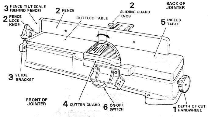
DEPTH OF CUT HANDWHEEL. Turning the handwheel counterclockwise will lower the infeed table to maximum depth of 1/8 in.
