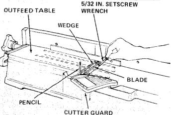
procedure under "REPLACING CUTTER BLADES" on pgs. 19 thru 21. 5. If a cutter blade adjustment is not required, check each locking screw of each wedge (5/32" setscrew wrench) and tighten if necessary. Hold the pulley
