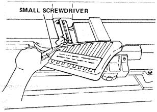
6. While holding cutterhead pulley firmly with one hand, gently pry up each wedge using a screwdriver . . . remove wedges and blades.
