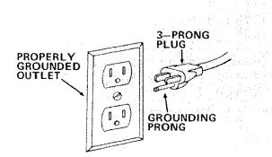
This power tool is equipped with a 3-conductor cord and grounding type plug which has a grounding prong listed by Underwriters' Laboratories Association. The ground conductor has a green jacket and is attached to the tool housing at one end and to the ground prong in the attachment plug at the other end.
