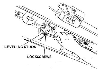
h. Loosen four lock screws 2 or 3 turns with 1/2 in. wrench.
