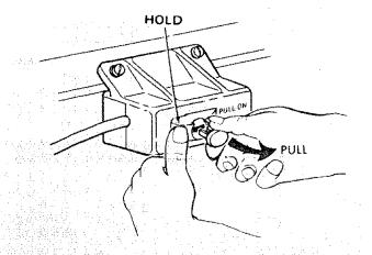
e. Plug motor cord into outlet in switch box.
