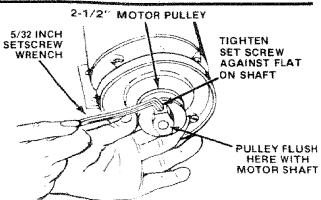
Install the 2-1/2" pulley onto the motor shaft and tighten the set screw in the pulley hub against the flat part of the motor shaft.
