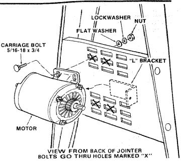
bracket so motor must be loosely assembled to bracket at this time.
