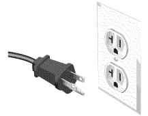
**NOTE:** Your Coffee Maker has a 3 prong grounded plug. To reduce the risk of electrical shock, this plug will fit in an outlet only one way. If the plug does not fit in the outlet, contact a qualified electrician. Do not modify the plug in any way.
