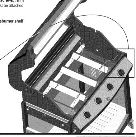
Place side shelf over right cart legs. Lip of shelf should fit between grill bottom and leg brace. Secure shelf brackets to cart legs using two 1/4-20x1/2" screws, 7mm lock washers, and 7mm flat washers on each bracket.
