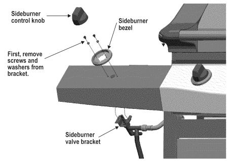
Insert sideburner into shelf, placing end of burner over sideburner valve. Valve should be in center hole of burner tube. Make sure pin on bottom of burner is in center hole in shelf bracket. Secure burner to bracket with two #10-24x3/8" screws, 5mm lock washers, and 5mm flat washers. See illustration below for correct burner-to-valve engagement.
