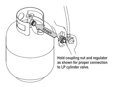
6. Turn the coupling nut clockwise and tighten to a full stop. The regulator will seal on the back-check feature in the LP cylinder valve, resulting in some resistance. An additional one-half to three-quarters turn is required to complete the connection. Tighten by hand only – do not use tools.
