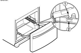
• Lower door into final position and tighten the screws ③.
