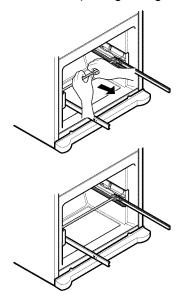
• Hook door supports ① into rail tabs ② on both sides.
