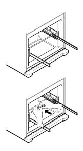
• With both hands hold the center bar and push it in to slide both rails in at the same time.
