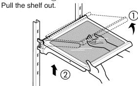
• To reinstall a shelf—Tilt the front of the shelf up and guide the shelf hooks into the slots at a desired height. Then lower the front of the shelf so that the hooks drop into the slots.
