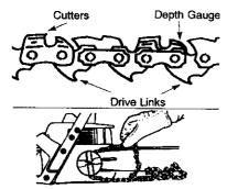
Place chain onto the sprocket Place chain over and behind clutch, fitting
