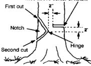
· After removing the wood from the notch, make the felling cut on the opposite side of make the reliing cut on the opposite side of the notch. This is done by making a cut about two inches higher than the center of the notch. This will leave enough uncut wood between the felling cut and the notch to form a hinge. This hinge will help pre-vent the tree from falling in the wrong direc-
