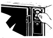
3. Set cooking times by turning the timer knob clockwise. Turn counterclockwise to reduce time.
