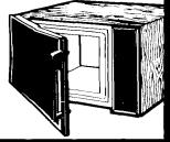
**DO NOT** operate the oven if it is damaged. It is particularly important that the oven door close properly and that there is no damage to the (1) Door (bent), (2) Hinges and latches
