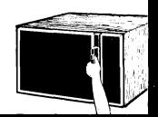
**DO NOT** attempt to operate this oven with the door open since open-door operation can result in harmful exposure to microwave energy. It is important not to defeat or tamper with the safety interlocks.
