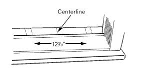
C Turn the bolts and tighten the lock nuts to make the sill supports level or tilt down 1/8" to the outside. Line up the "V" notch with 12%" marks. Drill pilot holes and attach the sill supports.
