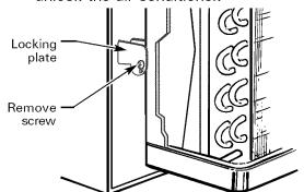
D Remove and discard the shipping screw on the back of the air conditioner to allow removal of the air conditioner from the case.
