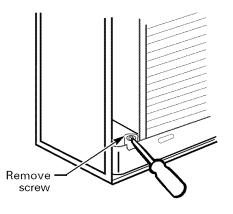
E Pull the bottom corners of the air conditioner and slide it out of the case.
