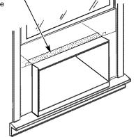
H Place the vinyl window gasket over the case top gasket. Insert the panel tabs through the slits in the gasket. Cut the gasket on each side to the width of the window.
