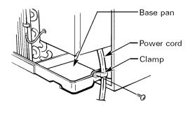
**C** When the wall outlet is to the left, extend the cord under the unit and hold it in place with the
