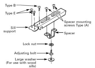
B Measure 12<sup>3</sup>/<sub>8</sub>" from the centerline on both sides for the sill support brackets.
