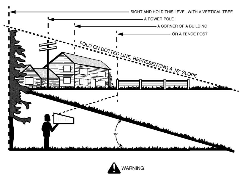
Do not mow on inclines with a slope in excess of 15 degrees (a rise of approximately 2-1/2 feet every 10 feet). A riding mower could overturn and cause serious injury. If operating a walk-behind mower on such a slope, it is extremely difficult to maintain your footing and you could slip, resulting in serious injury.
