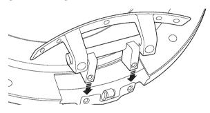
Fasten the hinge assembly to the edge using 2 machine screws (#8).
