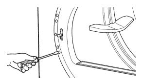
Switch the strike bracket and its cover on the opposite side by removing the screws. Reinstall both on the opposite side.
