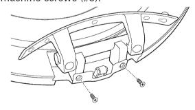
Hold the door on its side with one hand and fasten the remaining 2 screws as shown.
