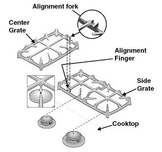
Place grate over the burners. Place the alignment fork of the center grate over the alignment finger of the side grates. Align the tips under each center of the grate to the holes on the burner caps. The tip should fit in the holes. Make sure that each tip fits in the burner cap of each of the front and rear burners.
