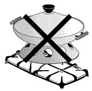
DO NOT use a wok if it is equipped with a metal ring that extends beyond the burner unit. Because this ring traps heat, the cooktop surface could be damaged.
