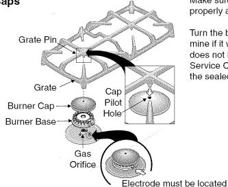
Make sure each burner cap is properly aligned and level.
