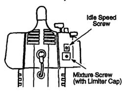
ADJUSTING PROCEDURE Idle Speed "IDLE"
