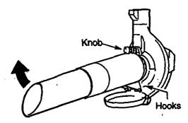
When converting back to the blower feature, make sure latch on the vacuum inlet cover is securely fastened.
