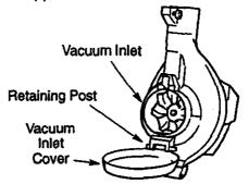
Place the hooks on the vacuum tube on the retaining posts; pivot tube into position. Secure vacuum tube by turning the knob clockwise until tight.
