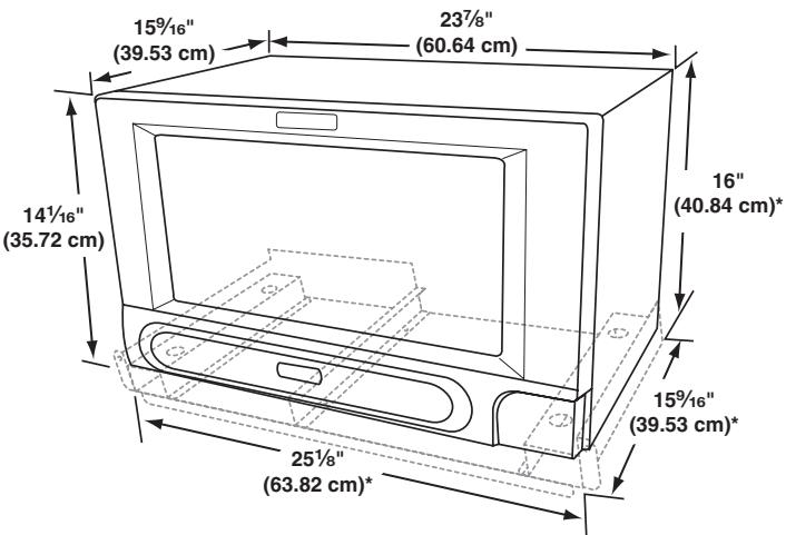
\*Measurements include bottom duct. Width does not include side flares of bottom duct.
