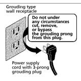
All models are equipped with appropriate 3-prong service plug to provide proper service and safe positive grounding. Do not change plug in any way. Do not use an adapter plug. If your present wall outlet does not match your plug, call a qualified electrician to make the necessary corrections. SAVE CARTON and these INSTALLATION INSTRUCTIONS for future reference. The carton is the best way to store unit during winter, or when not in use.
