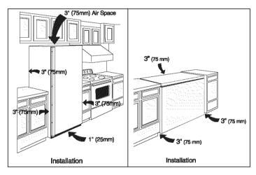
**NOTE:** The exterior walls of the freezer may become quite warm as the compressor works to transfer heat from the inside. Temperatures as much as 30° F warmer than room temperature can be expected. For this reason it is particularly important in hotter climates to allow enough space for air circulation around your freezer.
