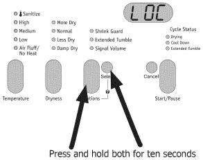
Press and hold both for ten seconds to lock or unlock the controls.
