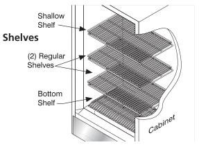
The appliance is provided with 4 shelves. One goes on the floor of the cabinet and the other 3 are placed in the metal side supports wherever they are needed. The shallow shelf goes in the upper position.
