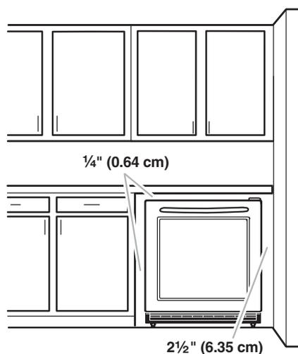
To ensure proper ventilation for your refrigerator, allow for a  $\frac{1}{4}$ " (0.64 cm) space on each side and at the top. When installing your refrigerator next to a fixed wall, leave 2 $\frac{1}{2}$ " (6.35 cm) minimum clearance on each side to allow for the door to swing open.
