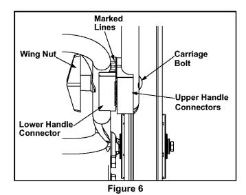
Secure the handle connectors in position by tightening each wing nut (carriage bolts must be seated properly into the handle and grooves must line up between connectors). Also make certain the bottom tip of the upper handle connector in front of the bottom tip of lower handle connector. See Figure 6.
