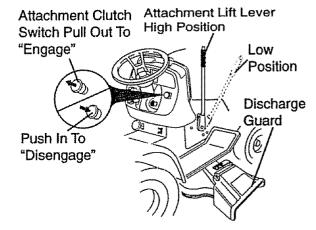
ACAUTION: Do not operate the mower without either the entire grass catcher, on mowers so equipped, or the discharge guard in place.
