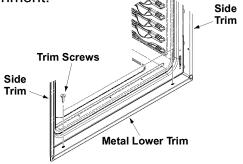
b. Using two trim screws provided, secure the bottom trim to the bottom edge of the cabinet.
