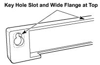
**c.** Match the key slot with the rivet on the bottom of the side trim, and lower the trim onto the rivet.
