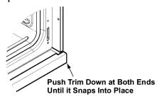
caution: Be sure you do not tip the oven forward during installation or you may bend the bottom trim. The bottom trim provides an opening for cooling air to enter the cabinet. This opening should never be blocked.
