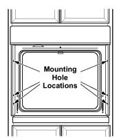
The screws must be a minimum of 1/4" from the front of the cutout.
